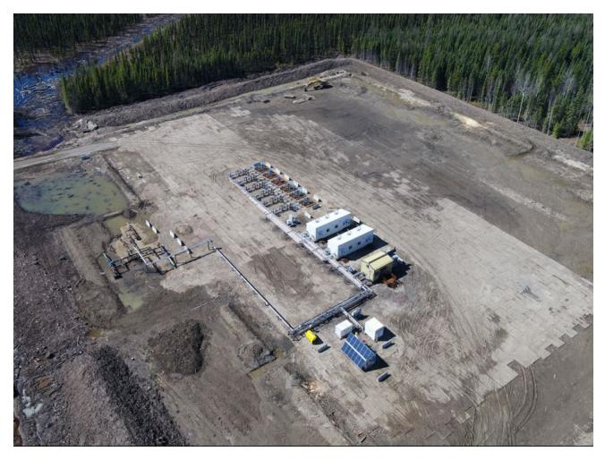
Located in the McKinley / Tony Creek field, near Fox Creek Alberta, the Shell trial well pad has 6 wells producing from the liquid rich Duvernay shale and uses gas lift for artificial lift.
