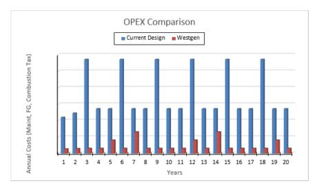
Eliminating the need for a load bank, coupled with the EPOD's partial duty cycle design and solar power input resulted in reduced fuel gas consumption by \$9,000 per year. The overall reduction in maintenance, fuel gas, and carbon tax resulted in more than 85% savings in operating expenses compared to the previous design.
